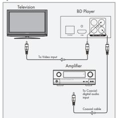
1 Connect a coaxial digital cable into the digital output »COAXIAL« on the back of the device and into the corresponding socket of the digital amplifier.
